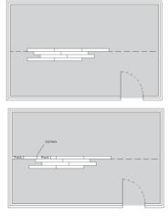
Score a line on the last plank then deep cut along the line. Continue this way until you have at least three rows complete. Mark pencil line along the last row and remove the planks keeping in the correct order for replacement. Ensure the area is clean and dust
